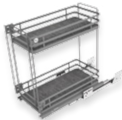
300 Base Pull Out 500 deep. To suit a 300 x 720 base cabinet. 30Kg loading. Code: STORANT0002
